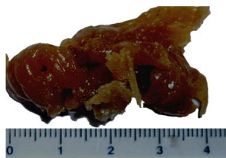
Figure I. 1: Browning in blend of LDPE + (E-C) processed at 160°C.
