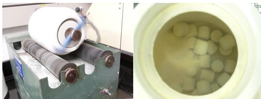
Figure 2.3: Ball mill used to diminish the bulk size of materials encapsulated in silica gel.
