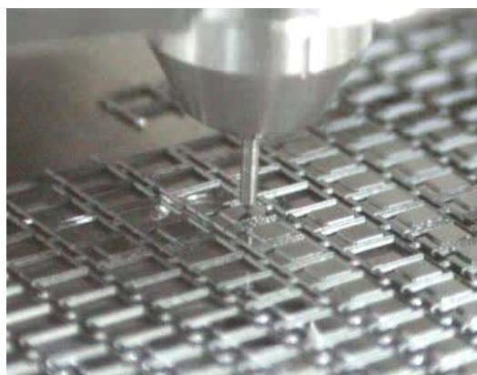
**Figure 1.** Functional indentation testing of accelerometer switch
