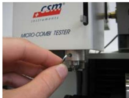
**Figure 11.** Easy change of indenter tip with CSM MHT
