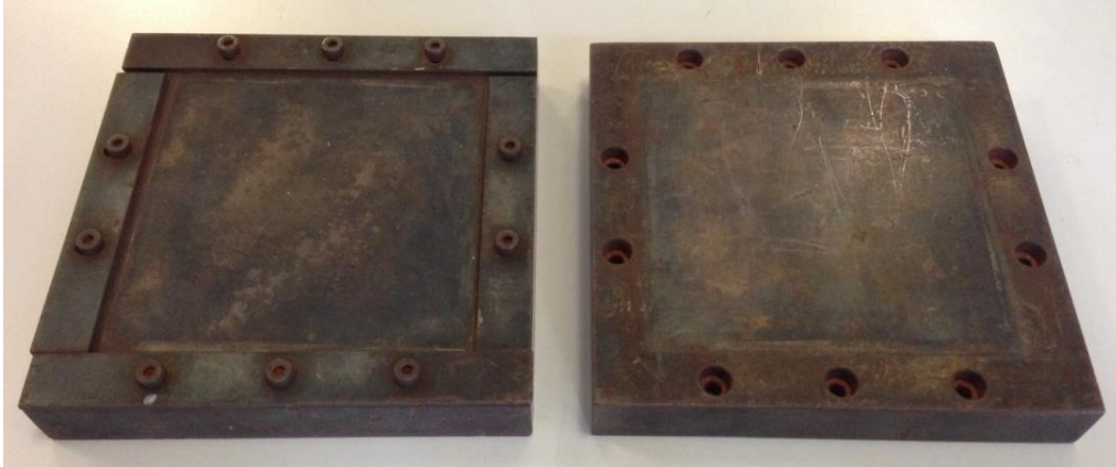
Fig. II.3 : Casing for the PEKK plates crystallization
