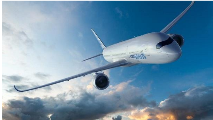
Fig. 1: Airbus A350 XWB with more than 50% by weight of composite in the structure
