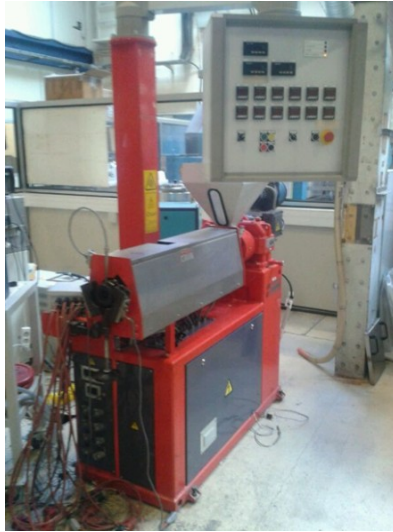
Figure 2.15 Extrudeuse monovis Mapre E1 30-33D
