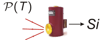
FIGURE : Illustration of the power receive by the detector and the associated output signal
